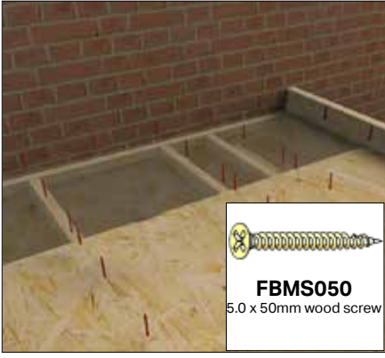
Use the screws provided to secure the board down into the firrings at 300mm centres.
