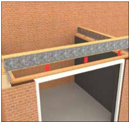
Position the front beam on to the structure and slot the male tenons into the female slots of the side beams. If you are only dealing with 2 beams, position the beam with the female end first. Support beam over any wide unsupported spans.
