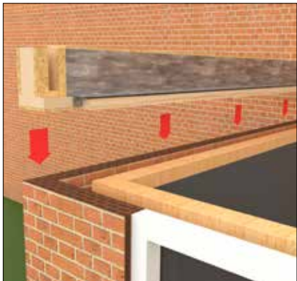
Take the female beam, lift the beam into position as per the above positioning depending on your situation. Prop if needed.
