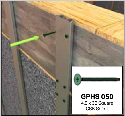
Detail Specific to hup! jobs. Fix the external clips into the wall panels and beams using 6x GPHS050 screws. Fix 4 of the screws into the beam, 2 at the top and 2 at the bottom. Fix the remaining 2 into the wall panel as shown. Do this on each box beam.
