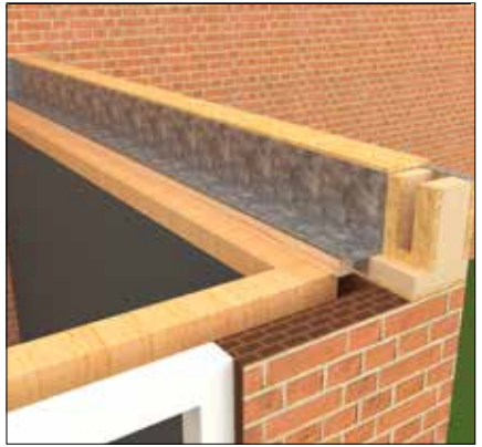
Align the opposing beam in the same way, lining beam up as above. Any gaps between the box beam and the host wall will be filled at a later stage.
